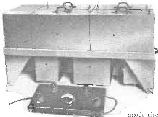
An experimental single-span receiver is shown here together with the remote control unit for magnetic tuning.
